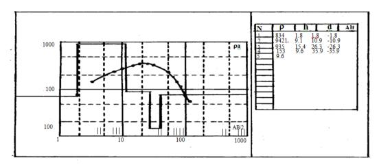
Fig 4: VES curve for resistivity data obtained at location 1
