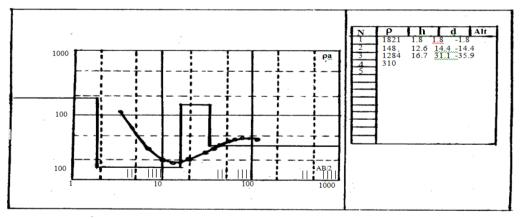
Fig 6: VES curve for resistivity data obtained at location 3
