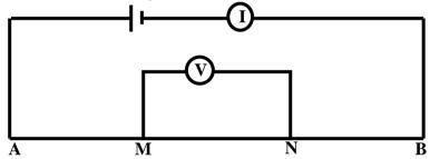
Fig 3: Schematic diagram of schlumberger array with potential (V) electrodes, M, N, inner and current (I) electrodes, A, B, outer.
